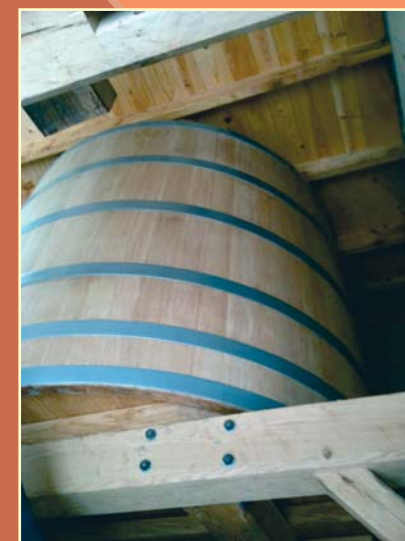
Ageing tank in a local cognac distillery
