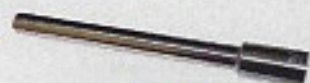
140663 Thermowell, Socket Weld, 3/4", 304SS, .260 bore, U-7 1/2", Straight -.75, OAL-9.25" c/w 1/2" NPT Instrument Connection
